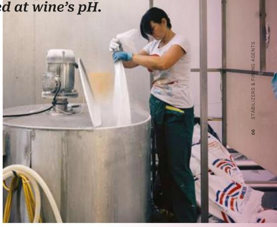
Proteins can be removed at this stage with Bentonite, color may be fine-tuned with carbon and tannins, tartrates stabilized with ion exchanging through the Stabymatic described in the equipment chapter. More modern technologies like Chitocel based technologies can also help with microbiological control and fining varous compounds including heavy metals. In the finished wine these treatments can be fine-tuned if needed.
