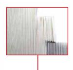
Filter elements are fluxed with extra pure water and then dehydrated with hot and sterile air flow.
