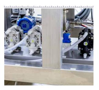
**REGENERANT DOSING PUMPS WITH SAFETY VALVES** Pneumatic valves for detergent supply for the system.
