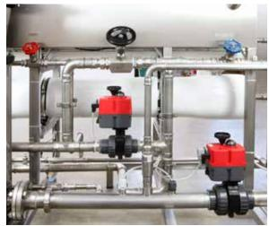
**MANUAL REGULATION VALVES**Allow the accurate control of the membrane pressure.
