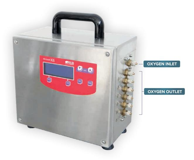
Microsafe X6 is an oxygenation system equipped with six delivery points, designed for all applications that don't require micro-dosing. It doses discontinuously, changing the delivery point every 10 minutes, cyclically repeating the oxygen dose every hour.
