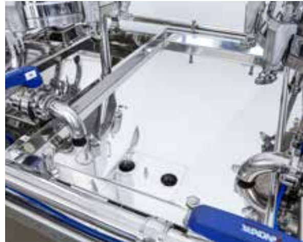
UNFILTERED OIL RECOVERY TANK
