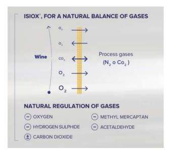
ISIOX technology enables the regulation of dissolved gases at the molecular level. The treated wine flows through a hydrophobic molecular sieve in counterflow to the technical process gas. The partial pressure difference results in the subtraction or addition of low molecular weight gases dissolved in the product. The system thereby provides the best alternative to stripping, preventing losses in aroma.
